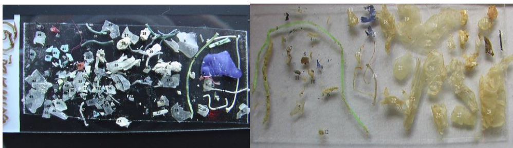
Figure 5. Suspected plastic particles in a sample from coastal water near Tumen River estuary prepared for spectra identification (4x magnification) (left) and suspected plastic particles in a sample from Razdolnaya/Suifenhe River prepared for spectra identification (4x magnification) (right).
