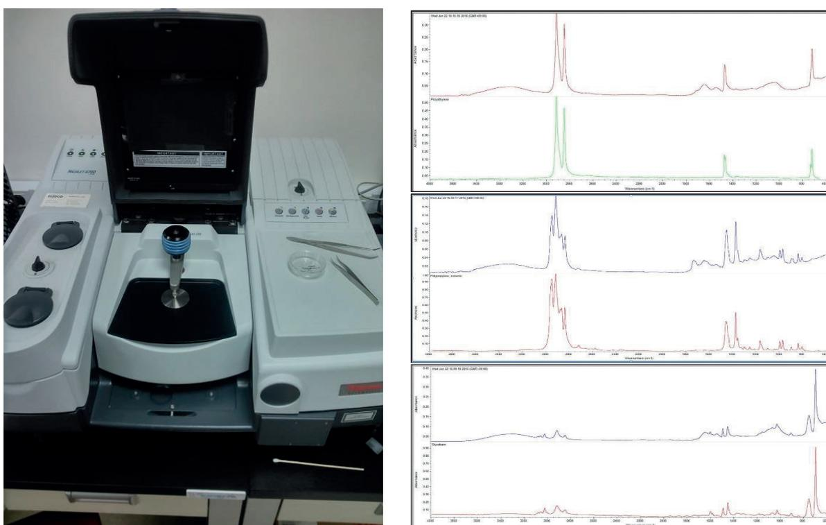
Fig.12. FTIR spectrometer and IR-spectra of the most frequent polymer types in the marine environment (Polyethylene(PE), Polypropylene (PP), and Polystyrene(PS)). Reference spectra of each polymer type are depicted below actual spectra of marine microplastics.
